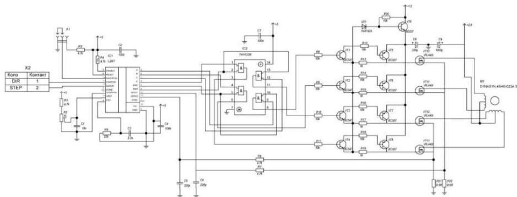
Fig. 2. Electrical diagram of the step motor driver
