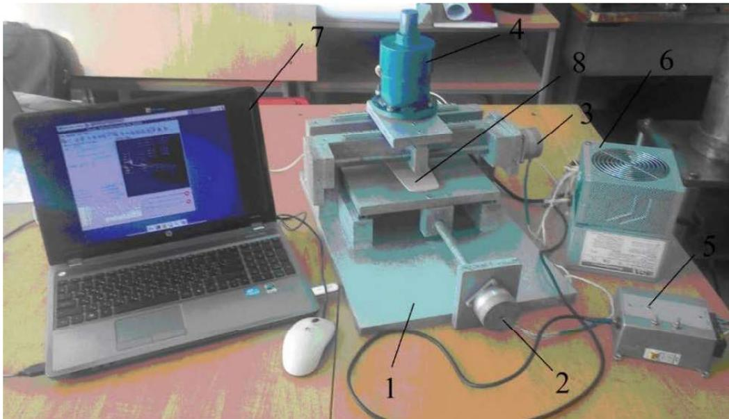
Fig. 5. General look of a machine with two-coordinate movement system for perforating parts of the top of the shoe: 1 - frame; 2-system of moving in coordinate Y; 3-system of moving along the coordinate X; 4-line electric motor; 5 – power and control supply of LEM; 6-stepper motor drive power supply; 7- electronic calculating machine (ECM); 8-detail
