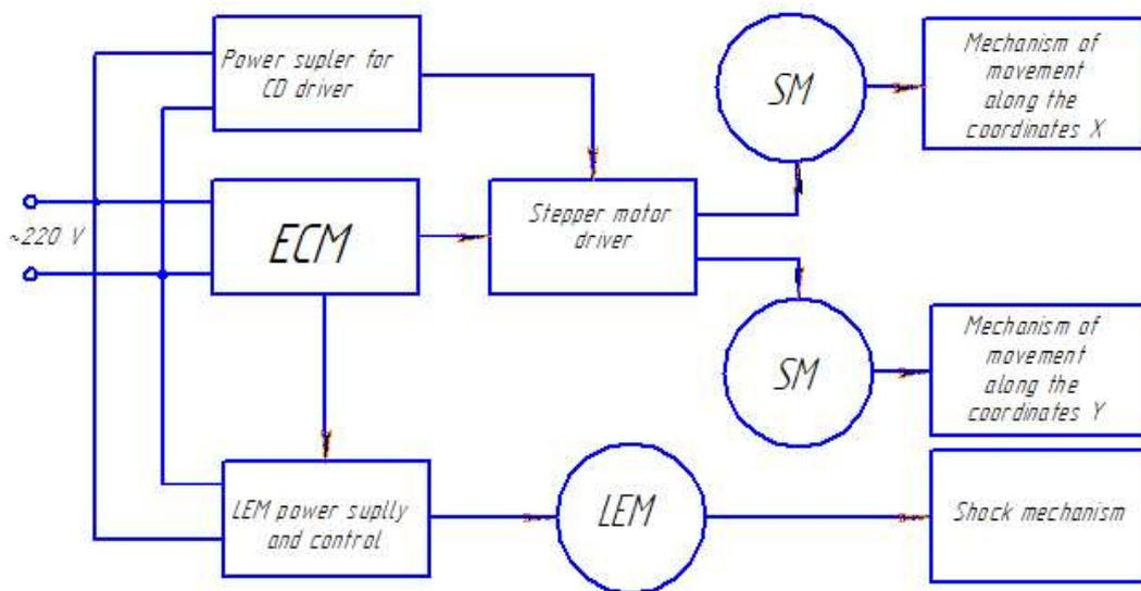
Fig. 1. Structural scheme device with two-coordinate movement system for impact perforation and marking of parts and products
